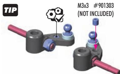
When using rearward hole, you can reinforce the steering block (for hard crashes) by installing an M3x3 setscrew in the forward hole.
