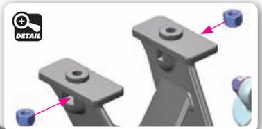
**TIP** 4x To tighten the setscrew you can also use the HUDY 17mm Wheel Nut Tool #107570.
