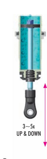
**2** Move the shock shaft up and down a few times to release the air bubbles trapped beneath the piston.
