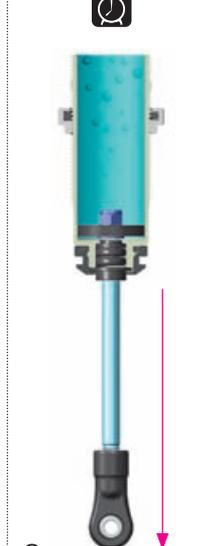
**3** Orient the filled shock vertically for several minutes with the shock shaft fully extended. The remaining air bubbles will release.
