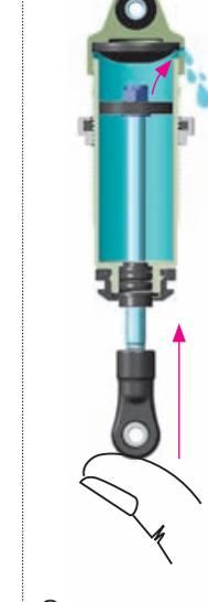
**6** Gently push the shock shaft completely into the shock body. Excess oil will flow through the hole in the shock cap.
