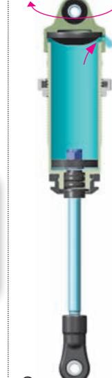
**5** Gently place the shock cap assembly onto the filled shock body. Excess oil will spill from the shock. Screw the shock cap onto the body by only a few turns.
