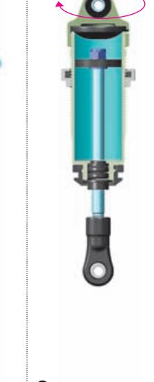
**7** Keep the shock shaft pushed in the shock body and tighten the shock cap completely. The rebound will be at approximately 0%.
